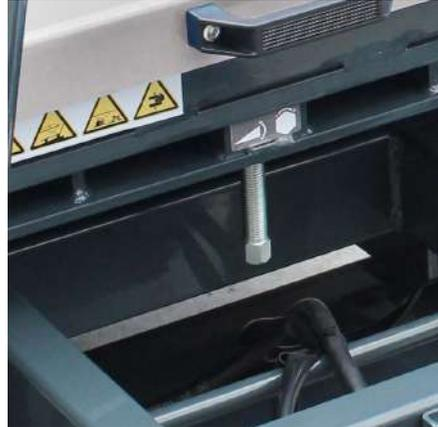
IL EST POSSIBLE D'AGIR SUR LA PLANÉITÉ DE LA TABLE  $\pm 3^\circ$
