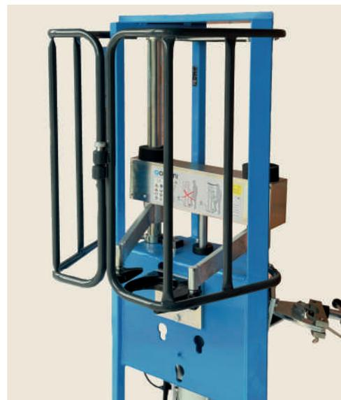
**SI LA GRILLE DE PROTECTION EST OUVERTE, LA MACHINE EST DOUÉE D'UNE SOUPAPE DE VERROUILLAGE DE SÉCURITÉ EMPÊCHANT LE FONCTIONNEMENT**
