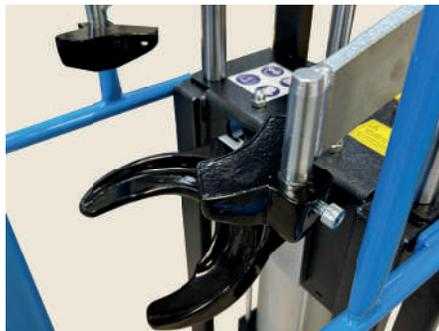
**LA MACHINE EST FOURNIE AVEC COUPELLE POUR LE BLOCAGE DU RESSORT Ø105 - 185 mm**
