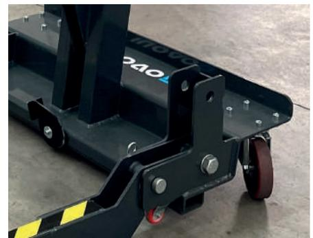
LES ROUES ARRIÈRE SONT PIVOTANTES POUR GARANTIR UNE MANIABILITÉ MAXIMALE
