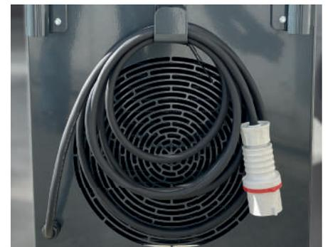
CÂBLE D'ALIMENTATION AVEC FICHE À 4 BROCHES À L'ARRIÈRE DE LA MACHINE
